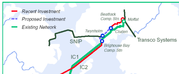
Figure 1 Possible solutions for Pipeline Cluden-Brighthouse Bay [15].
